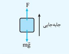
$$W_F = Fd \cos(0^\circ) = 20 \text{ (N)} \times 2 \text{ (m)} \times 1 = 60 \text{ J}$$
