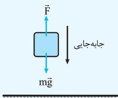
$$W_F = Fd \cos(180^\circ) = 20 \text{ (N)} \times 2 \text{ (m)} \times (-1) = -60 \text{ J}$$
