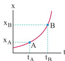
$$|\vec{v}_{av}|_{A,B} = \frac{\Delta x_{A,B}}{\Delta t_{A,B}} = \frac{x_B - x_A}{t_B - t_A}$$
