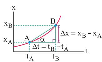
$$\tan \alpha = \frac{\text{مقابل}}{\text{مجاور}} = \frac{x_B - x_A}{t_B - t_A} = \frac{\Delta x}{\Delta t} = |\vec{v}_{av}| = AB$$
