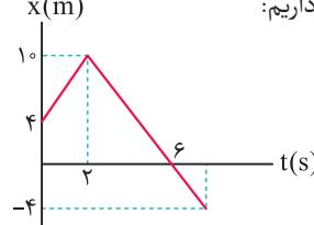
$$v = v_{av} = \frac{\Delta x}{\Delta t} = \frac{x_6 - x_2}{t_6 - t_2} = \frac{10 - 4}{6 - 2} = -2.5\text{ m/s}$$
