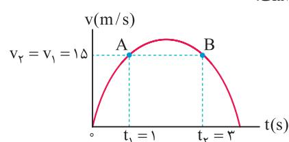
$$|\vec{a}_{av}| = \frac{v_2 - v_1}{t_2 - t_1} = \frac{15 - 15}{3 - 1} = 0$$
