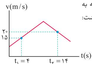
$$\begin{cases} t_1 = 4 \text{ s} \rightarrow v_1 = 15 \text{ m/s} \\ t_2 = 14 \text{ s} \rightarrow v_2 = 20 \text{ m/s} \end{cases} \Rightarrow a_{av} = \frac{v_2 - v_1}{t_2 - t_1} = \frac{20 - 15}{14 - 4} = \frac{1}{2} \text{ m/s}^2 = 0.5 \text{ m/s}^2 \Rightarrow \vec{a}_{av} = 0.5 \hat{i}$$
