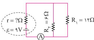
$$R_{eq} = \frac{R_1 R_2}{R_1 + R_2} = \frac{12 \times 6}{12 + 6} = 4\Omega$$
