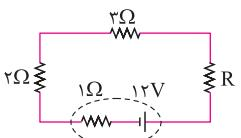
$$R_{eq} = R_1 + R_2 + R_3 \Rightarrow 11 = 2 + 3 + R \Rightarrow R = 6\Omega$$
